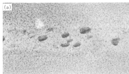
Figure 4 Variation in hydrogen bubble contrast on tilting (Alloy 7) after similar thin foil exposure as in Fig. 3. (a) BF g = 111, s \neq 0 (b) BF g = 444, s = 0 (c) BF g = 220, s + ve .
